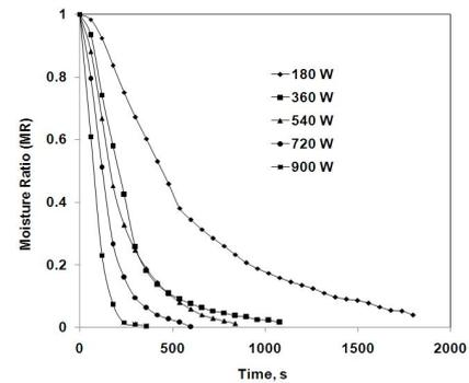
Figure 1. Moisture ratio vs drying time at various microwave powers
