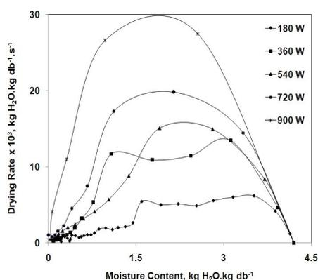
Figure 3. Drying rate vs moisture content at different microwave powers
