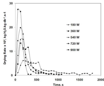
Figure 2. Drying rate vs drying time at different microwave powers
